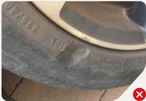
Tyre sidewall damage is not acceptable.
