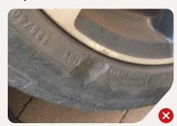
Tyre sidewall damage is not acceptable.
