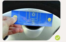
Scuffs to wheels totalling up to 50mm on the total circumference of the wheel trim, and on alloy wheels, are acceptable.
